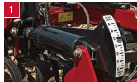
Hydraulic fore/aft control: maintain consistent agronomic output
