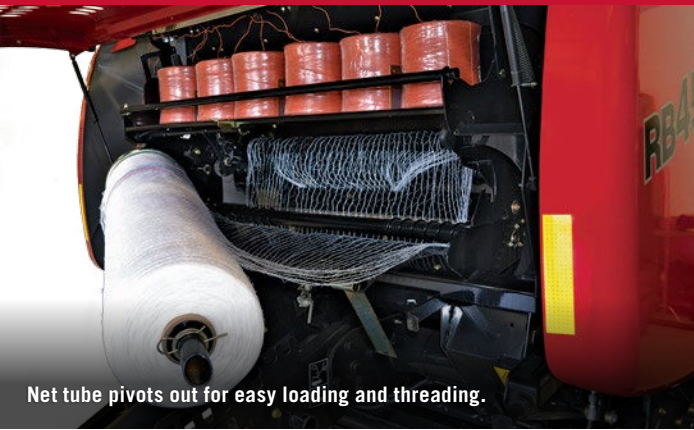
This baler is ready to bale with either net or twine. If twine is not being used, a spare net wrap roll may be stored in place of the twine balls.
