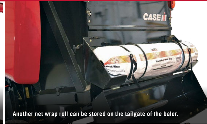
This baler is ready to bale with either net or twine. If twine is not being used, a spare net wrap roll may be stored in place of the twine balls.
