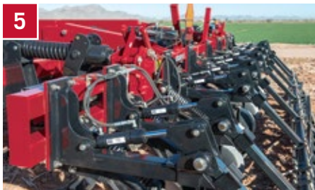
5 Crumbler pressure: achieve consistent clod sizing
