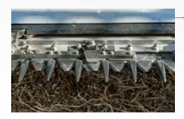
More robust knife heads include a factory-assembled and lubed knife arm and head vertically mounted, allowing adjustments as required to obtain the proper gearbox-to-cutterbar spacing.
