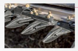
■ Knife heads, spline blocks, knife arms and hardware have been substantially beefed up to improve reliability and durability.
