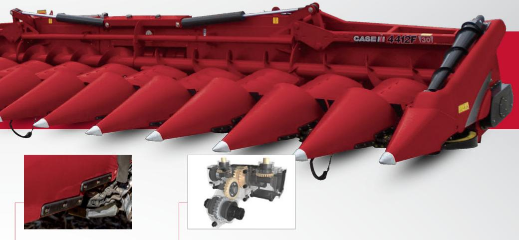
Replaceable wear strips are easy to service, keeping you in the field during optimal harvest windows.
