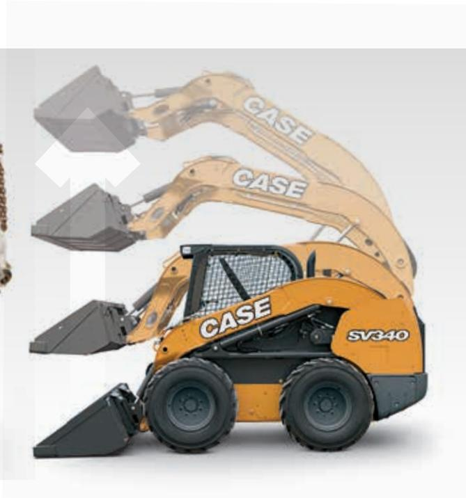
Vertical-lift machines are engineered for lift-and-carry and truck-loading jobs. The geometry of the dual arm allows the load to rise directly up, providing maximum reach at full height. Vertical-lift machines are ideal for reaching over the side of and into the middle of high-side trucks.
