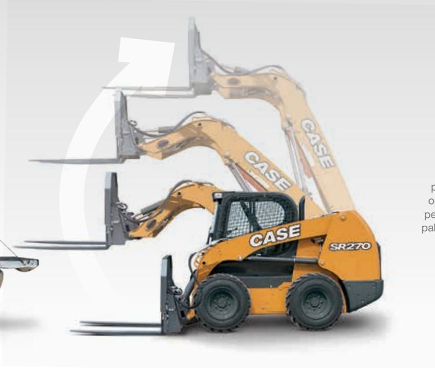
Radial-lift machines are engineered for digging, prying and pushing. The angle of the arm ties directly into the chassis for superior strength when digging and pushing. It also provides maximum reach at the operator's head height, making it perfect for loading and unloading pallets from trucks.
