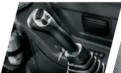
ERGONOMIC JOYSTICK Ergonomically designed joysticks reduce operator fatigue during the workday.
