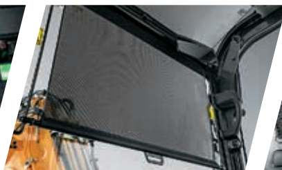
ROLLER SHADE A large upper roof glass provides additional visibility and a roller shade is provided to reduce glare and sunlight.
