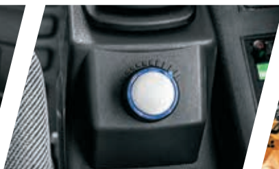
ACCELERATION DIAL WITH LED LIGHT The acceleration dial is easy to control and recognizable in dark working conditions thanks to an LED light.
